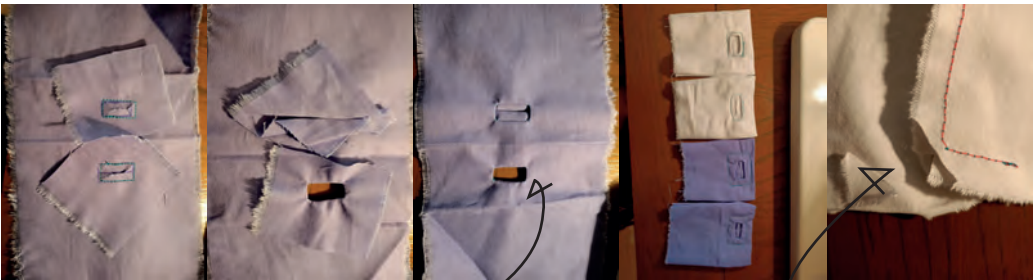
Making piped button holes that align & cutting extra fabrics for sharp corners.
